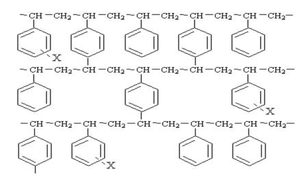
Figure 2.1: Polystyrene-divinylbenzene copolymer resin.
