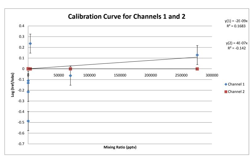
From the calibration curves performed on the LOPAP it can be seen that the calibration curve of channel 1 is relatively close to the expected, however the curve for channel 2 is very close to zero, which comes from very low concentrations of  $NO_2$  ions coming towards the channel 2 absorption. Even though the expected trend is present, that the slope of channel 1 calibration
